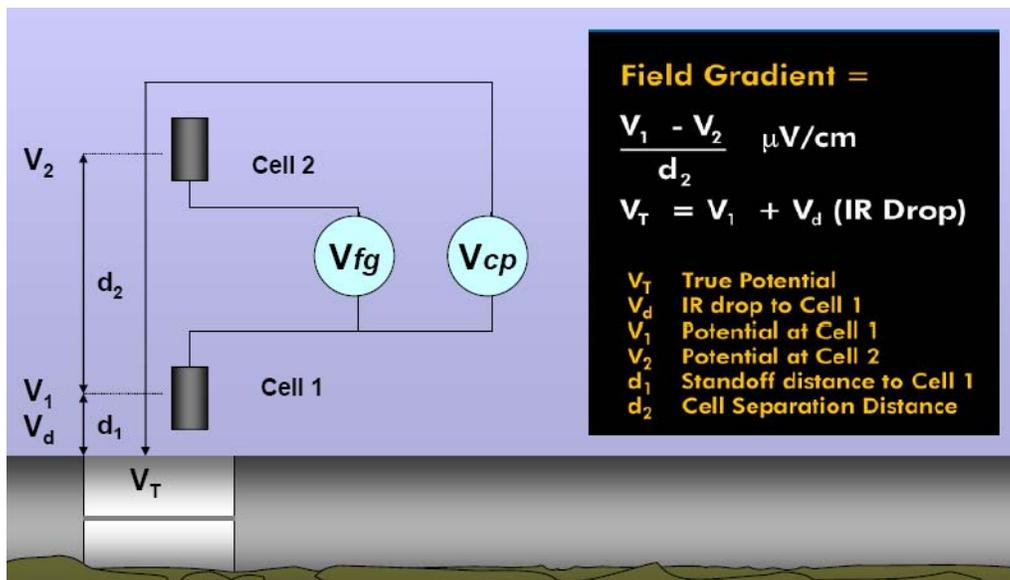
How field gradient is calculated from the potentials measured in the twin half cell probe
