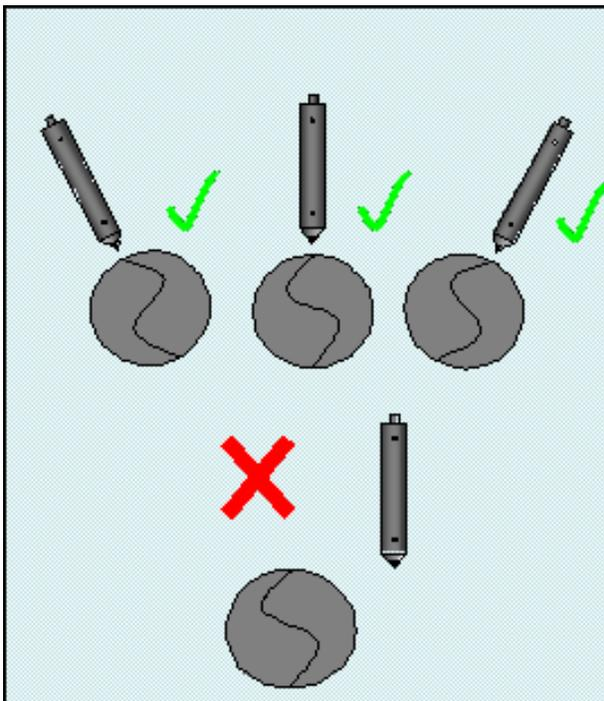
The probe should be aligned radially to the pipeline as shown above.
