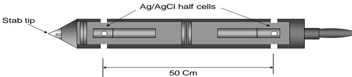
Example of twin half cell contact probe.
